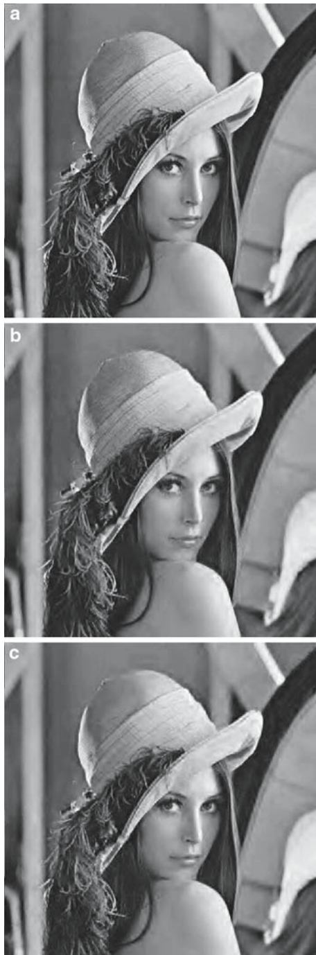
Fig. 5 The simulation results on Lena at 0.5 bpp by exploiting the proposed DD-MDC. a Both channels are available (36.25 dB). b Only channel 1 is available (32.74 dB). c Only channel 2 is available (32.34 dB)
